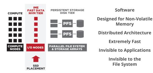
IME manages at-scale flash to eliminate file system bottlenecks and the burden of creating and maintaining application-specific optimizations. It delivers:
