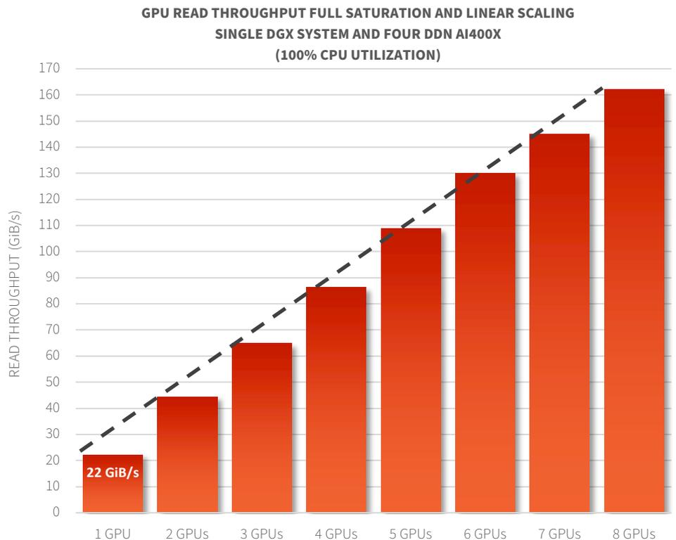
Figure 11. DDN A<sup>3</sup>I with GDS GPU throughput scaling on DGX system
