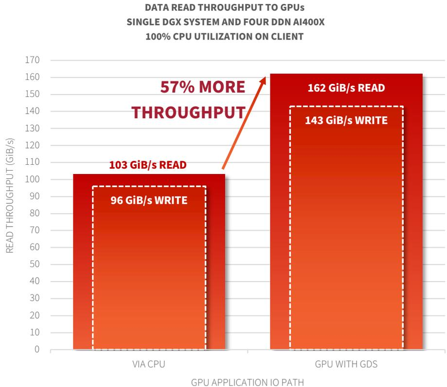
Figure 10. DDN A<sup>3</sup>I with GDS increased throughput performance on DGX system
