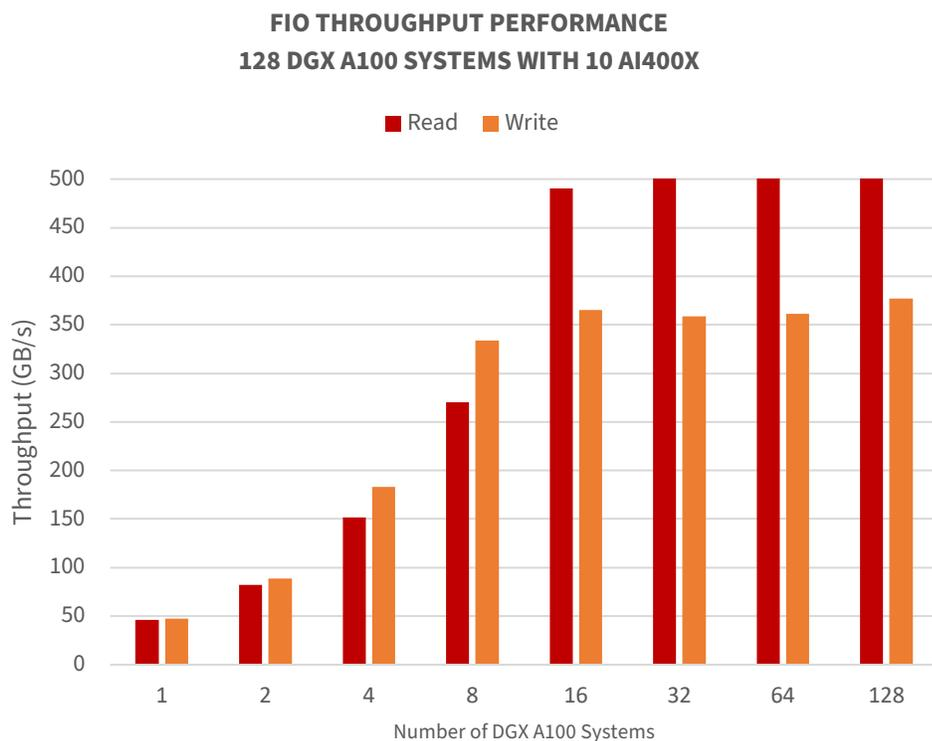
Figure 4. FIO throughput scaling with a very large number of DGX A100 systems
