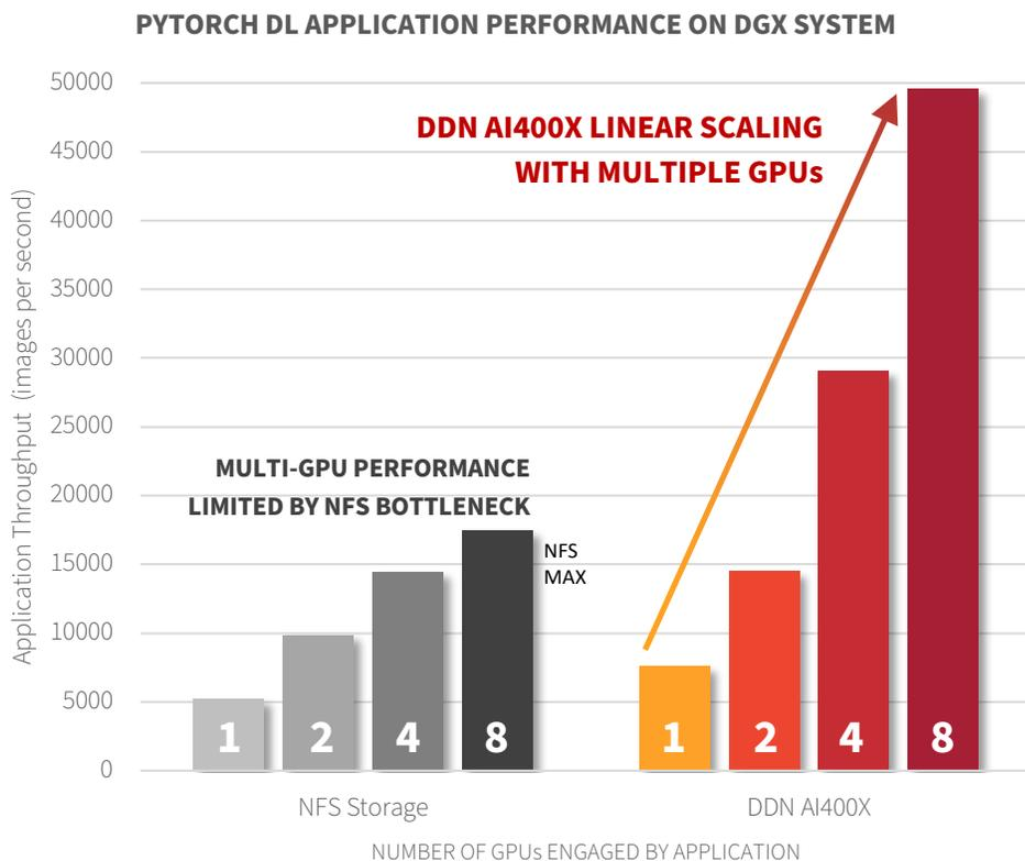
Figure 7. Scaling PyTorch application performance on DGX system
